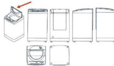
Set of drawings showing the industrial design in different states, with the perspective view in the open state while the projections show the design in the closed state
